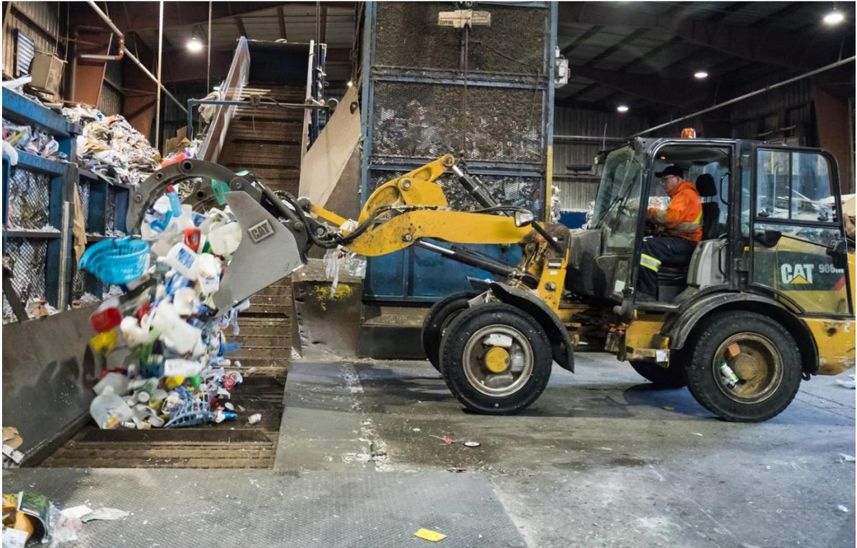
TRENTON, Ont. (01/12/20) – Billy, a sorter at [Quinte Waste Solutions](#), uses a loader to dump clean HDPE (high-density polyethylene) plastics onto a conveyor belt in Trenton on Monday Nov. 30, 2020. These plastics will go into a bale compactor that will press these plastics into specific bales that will be sold to companies that will reuse the material. Photo by Alex Bowman
